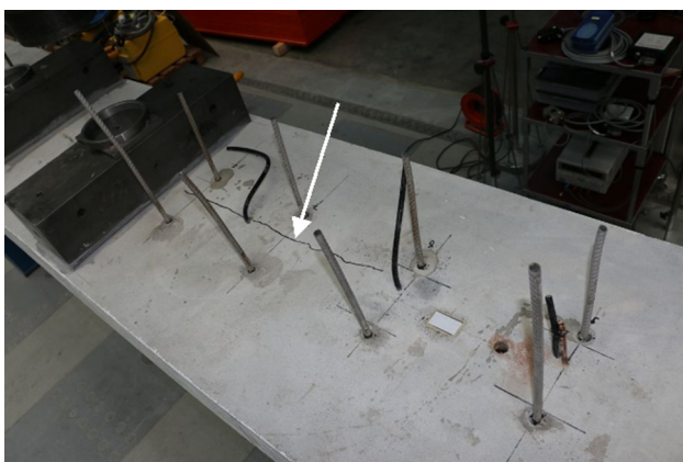
Fig. 19. Beam 5: only one longitudinal crack on the right beam top side (the side with no shear failure).
