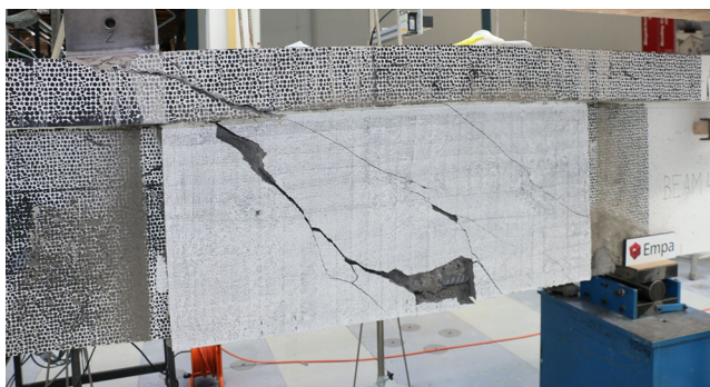
Fig. 23. Failure mode of Beam 4.
