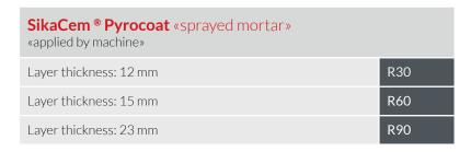
The fire protection measures and stated layer thicknesses are guide values and must also conform and be compatible with all relevant local regulations and standards
